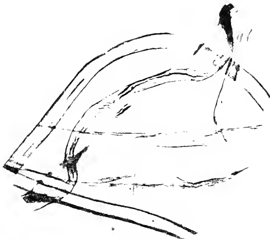
FIG. 2.—Cotton cellulose fibres \times 250 .
